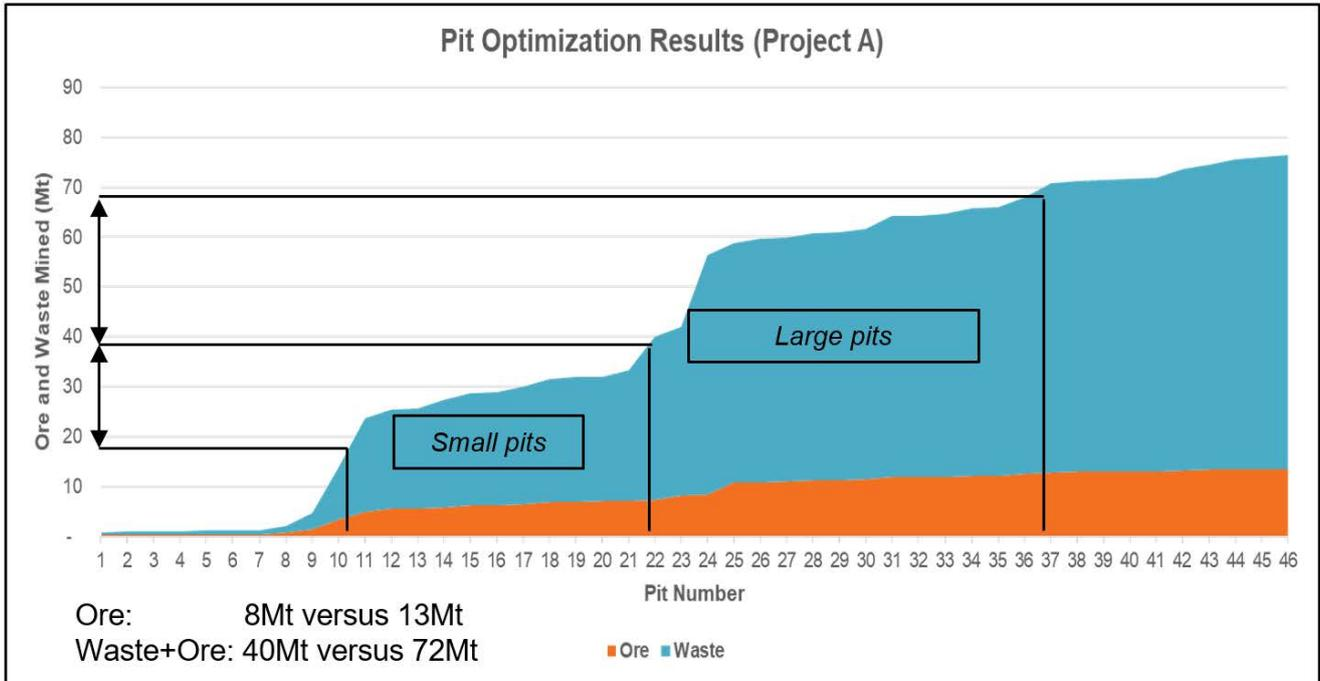
Figure 3 ore and waste mined for Project A
