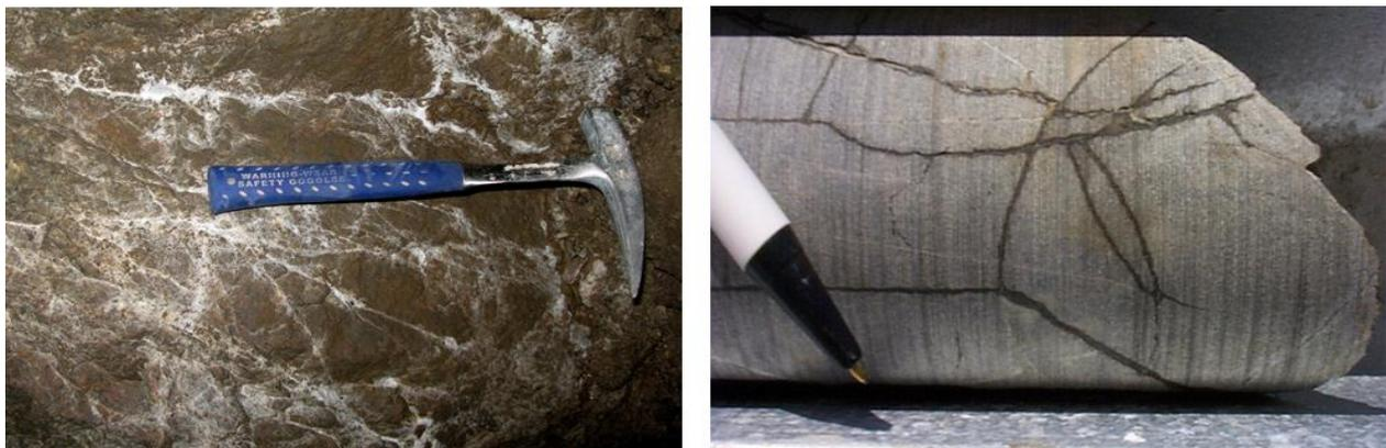
**Figure 7 Precipitated secondary minerals reveal degree of micro fracturing in Chilean porphyry and moisture enhanced micro fracturing from E 48 mine in Australia**
