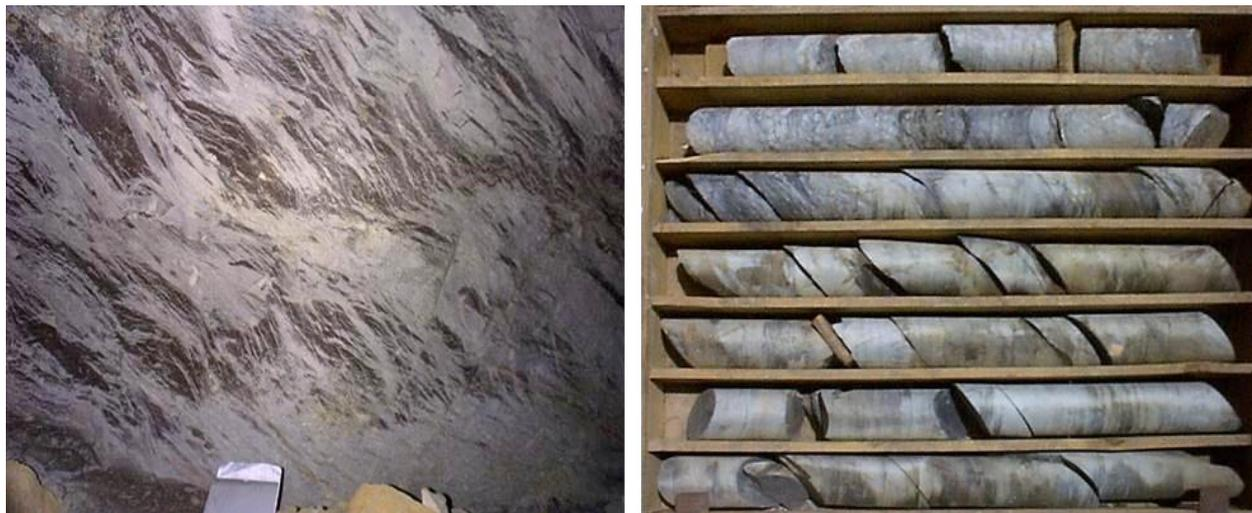
**Figure 4 Highly foliated metamorphic rock in this example from Aljustrel Mine in Portugal is e still very strong and exhibit relatively low strength anisotropy**
