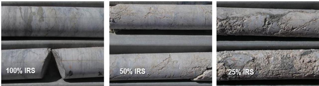
**Figure 8 Examples of high density of micro defects. The defects in the photo on the left, although numerous, have no effect on IRS; while defects in the photo in the middle and on the right dramatically reduce IRS**
