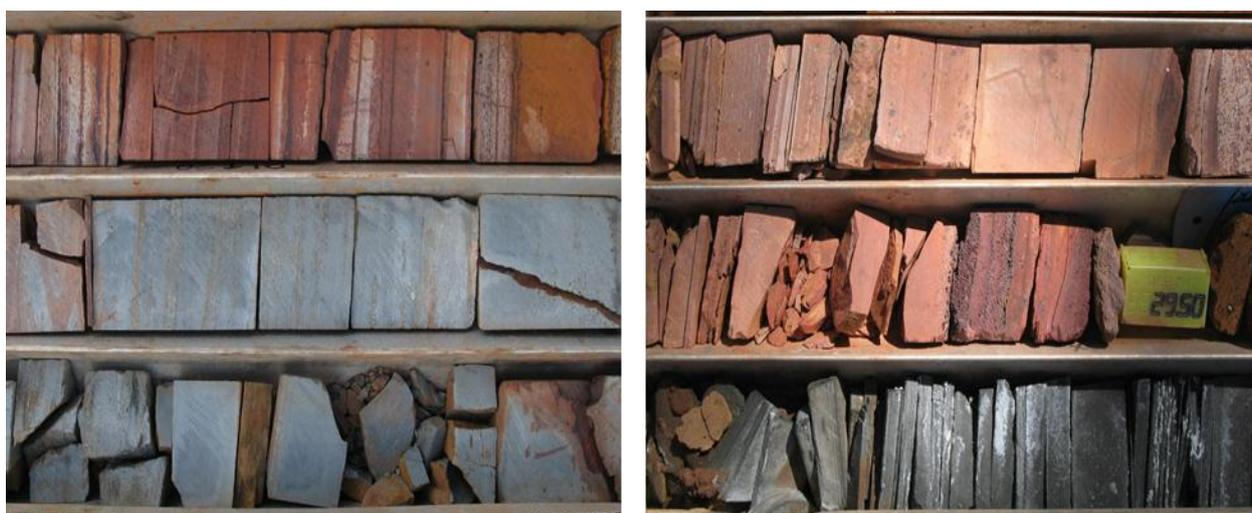
**Figure 5 The bedding planes in sedimentary rocks from Congo shows moderate rock mass strength reduction (left), but very low strength near the fault (right)**
