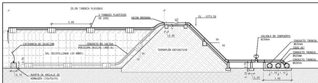
Figure 7. Typical cross-section of the starter embankment on the disposal spine side of a facility.
