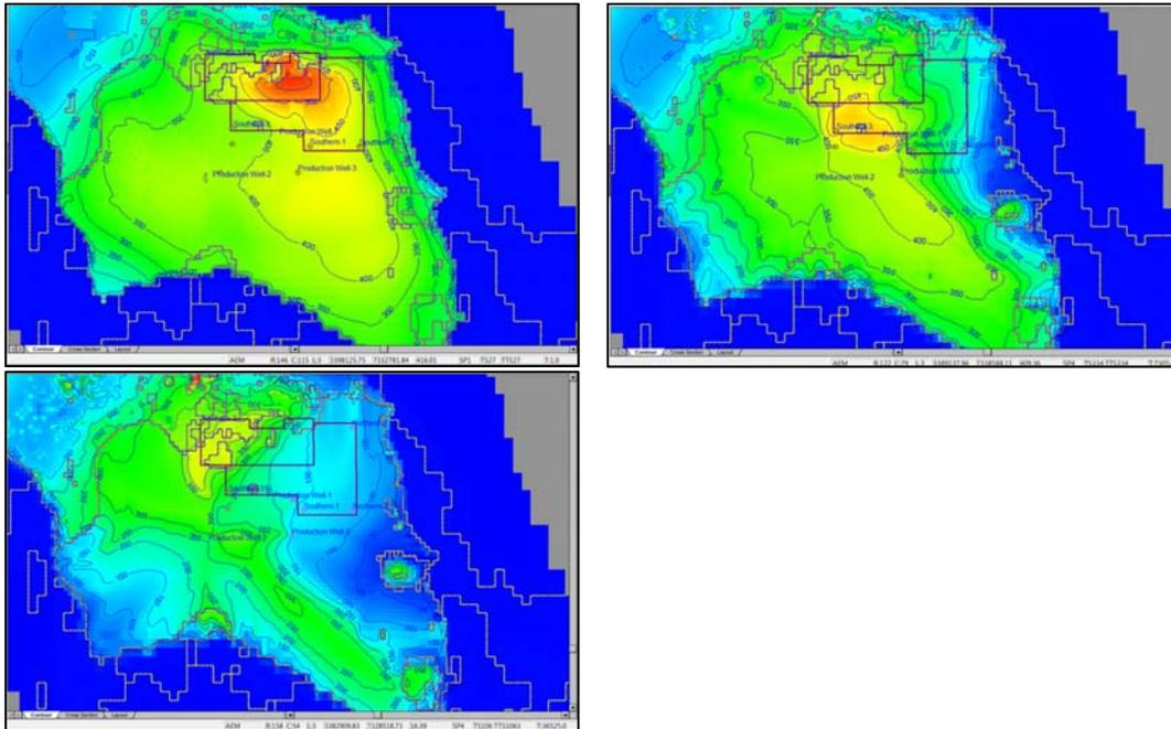
Figure 3.  $\text{Li}^+$  concentration evolution through production for a project in the lithium triangle -situation before production start and after 20 and 100 years of production – SRK Consulting (2016b)
