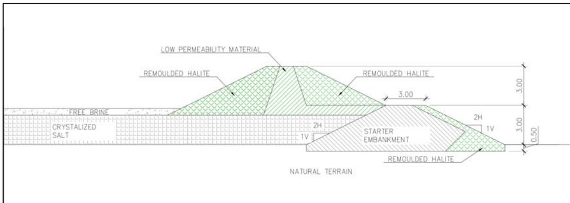
Figure 6. Typical cross section of a evaporation pond-salt stack for a project in the lithium triangle – internal database, SRK.
