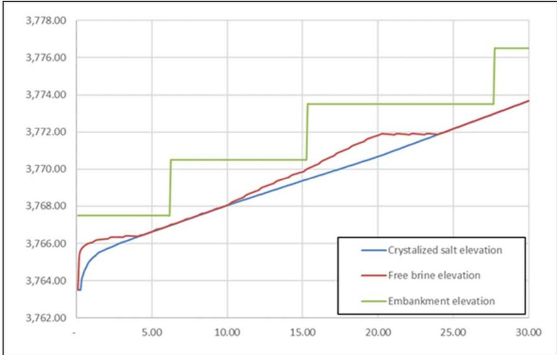
Figure 5. Brine storage level, crystallized salt elevation and embankment raising evolution over time for a project in the lithium triangle – internal database, SRK.
