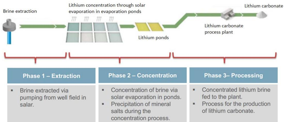
Figure 1. Conventional solar evaporation process flowchart – from Lithium Americas 2017.
