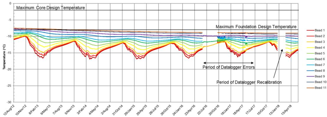
Figure 6b. Time series data for the key trench vertical GTC at chainage 0+085 m (ND-VTS-085-KT).
