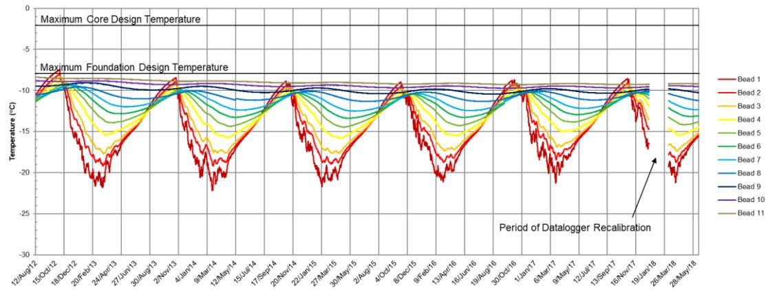
Figure 6a. Time series data for the key trench vertical GTC at chainage 0+040 m (ND-VTS-040-KT).
