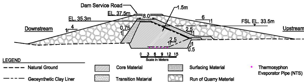
Figure 2. Typical design cross-section of the North Dam.
