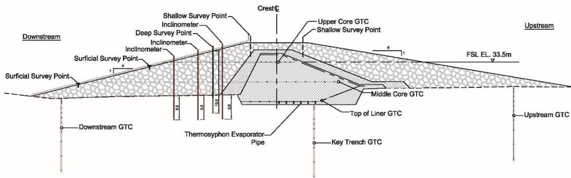
Figure 4: North Dam typical instrumentation.
