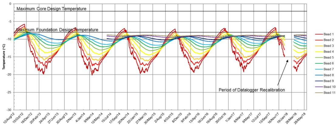
Figure 6c. Time series data for the key trench vertical GTC at chainage 0+175 m (ND-VTS-175-KT).
