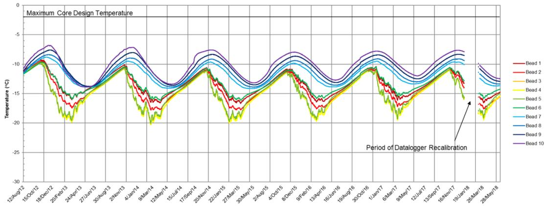
Figure 5c. Lower horizontal GTC at chainage 0+130 m, located at elevation 28.8 m (ND-HTS-130-28.8).
