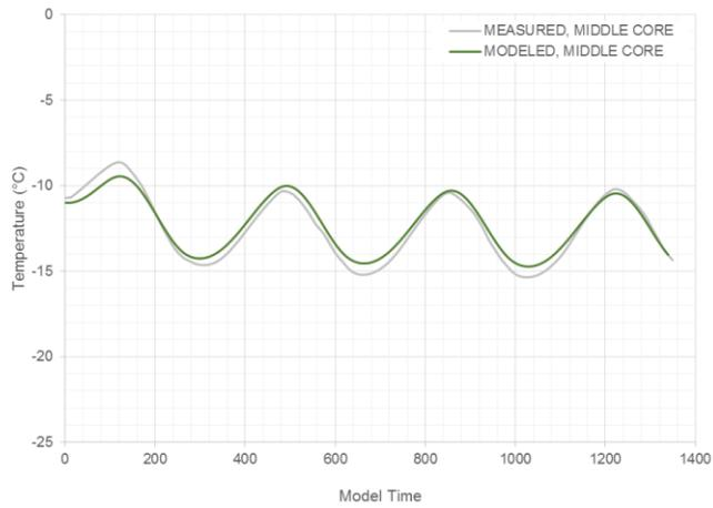
Figure 8b: Middle core temperature calibration model at chainage 0+085 m.
