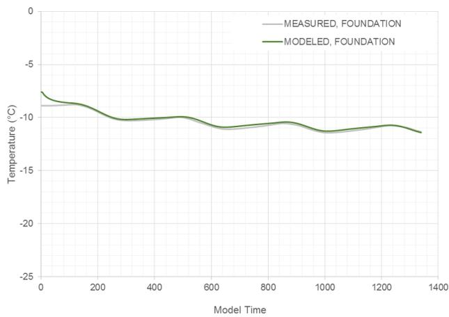
Figure 8c: Foundation temperature calibration model at chainage 0+085 m.
