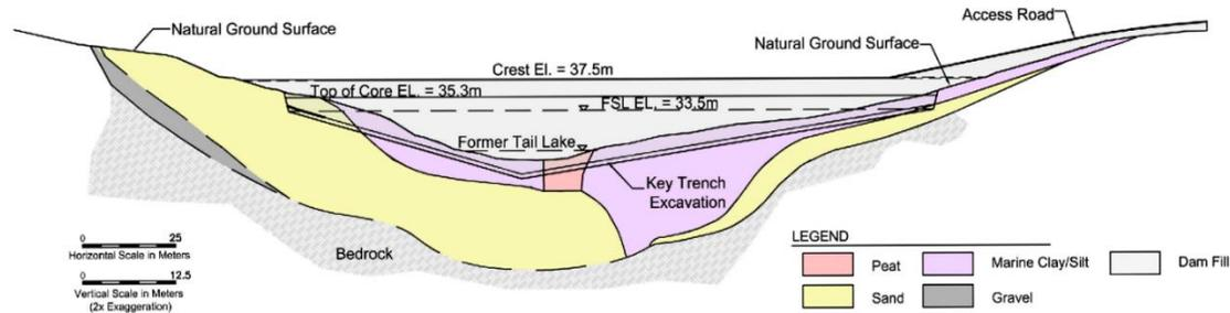
Figure 1. Longitudinal section of the North Dam showing generalized foundation conditions.
