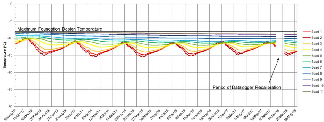
Figure 7b. Time series data for the key trench vertical GTC at chainage 0+130 m (ND-VTS-130-KT).
