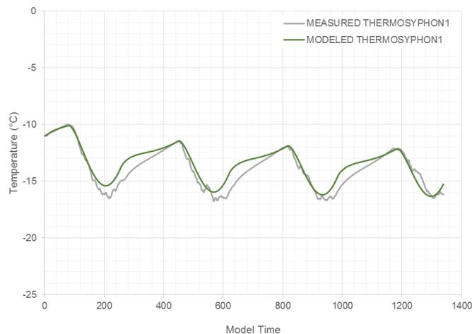
Figure 8a: Thermosyphon evaporator pipe temperature calibration model at chainage 0+085 m.
