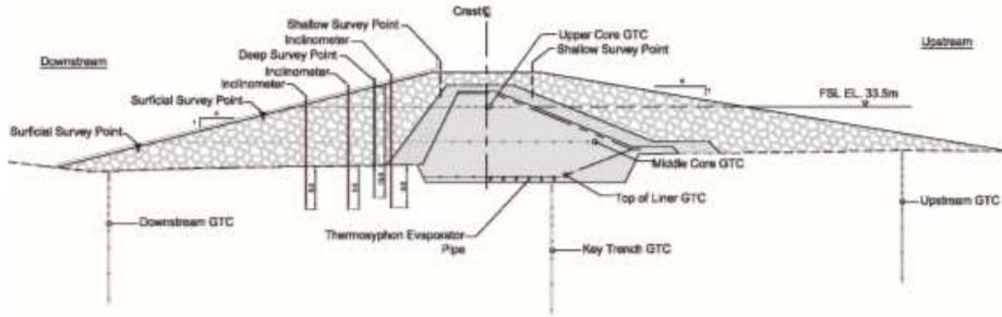
Figure 4. North Dam typical instrumentation.
