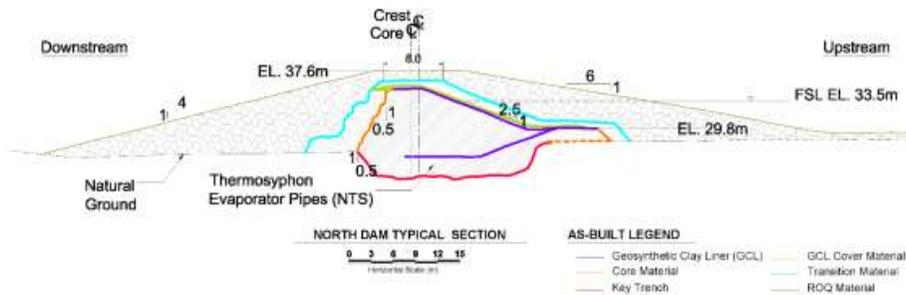
Figure 3. Typical as-built cross section of the North Dam.
