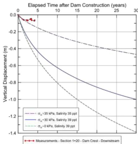
Figure 6: Vertical displacement history of the core crest.
