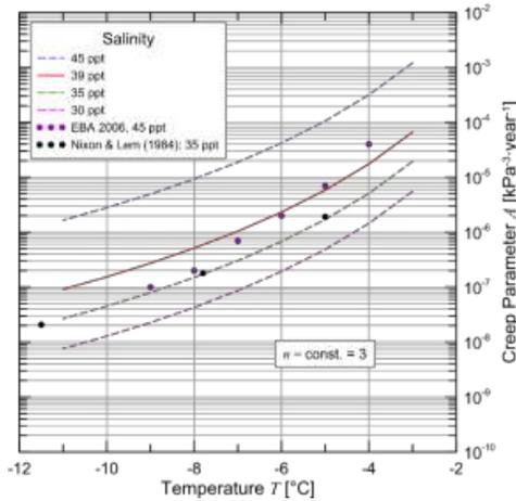
Figure 5: Creep parameter A for the marine clayey silt foundation material.
