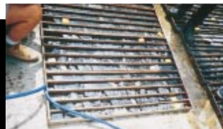
Inspection of diamond drill core and checking for core recovery
